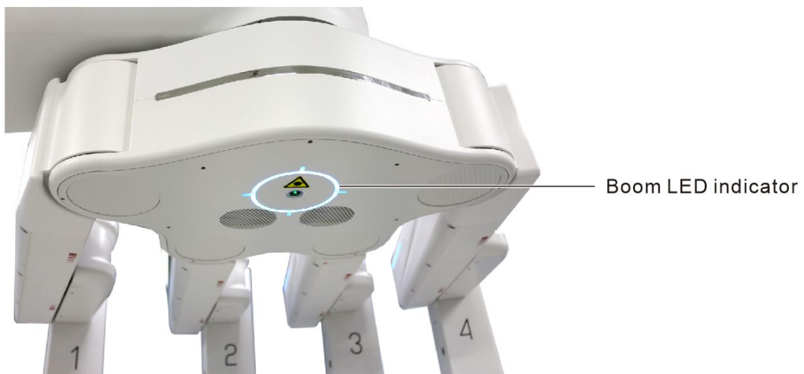
Figure 9.4 Boom LED Indicator
