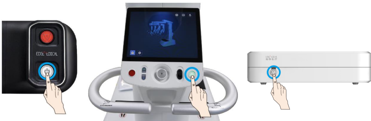
Figure 5.1 Power Buttons (from Left to Right: Surgeon Console, Patient Cart, Signal Distributor)
