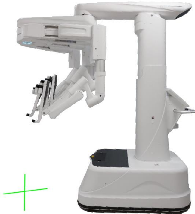
Figure 9.7 Positioning Laser Lines
