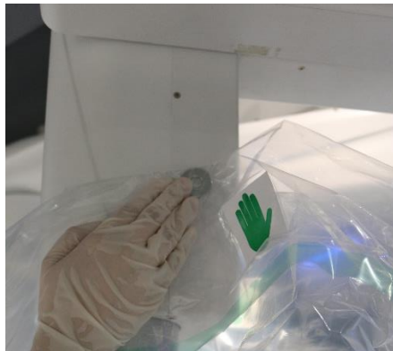
Figure 6.6 Attach Metal Discs to the Column
